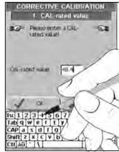
Left Fig: Display CAL-rated value after entering the foil/coating thickness.
