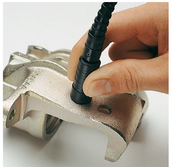
Measuring on rough surfaces, Zn/Fe with the ESD20Zn probe
